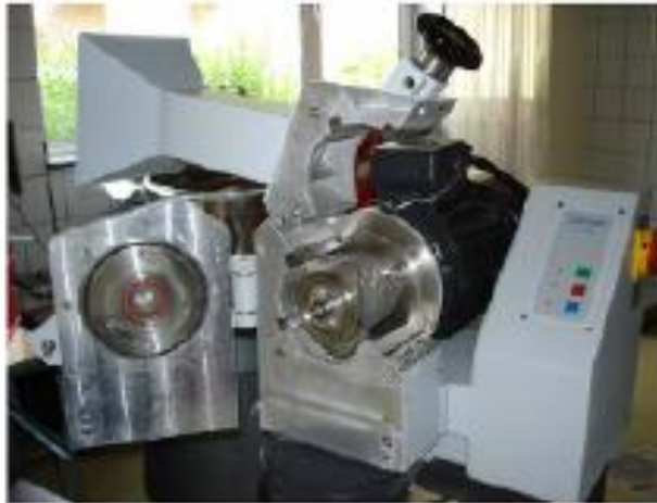
Retsch heavy duty cutting mill with hardmetal cutting inserts
