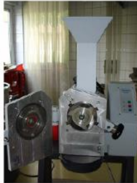
Retsch heavy duty cutting mill with hardmetal cutting inserts
